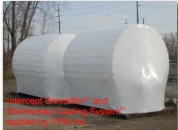
Intercept Technology Shrink Film protects large equipment from corrosion or rust during plant closing.
